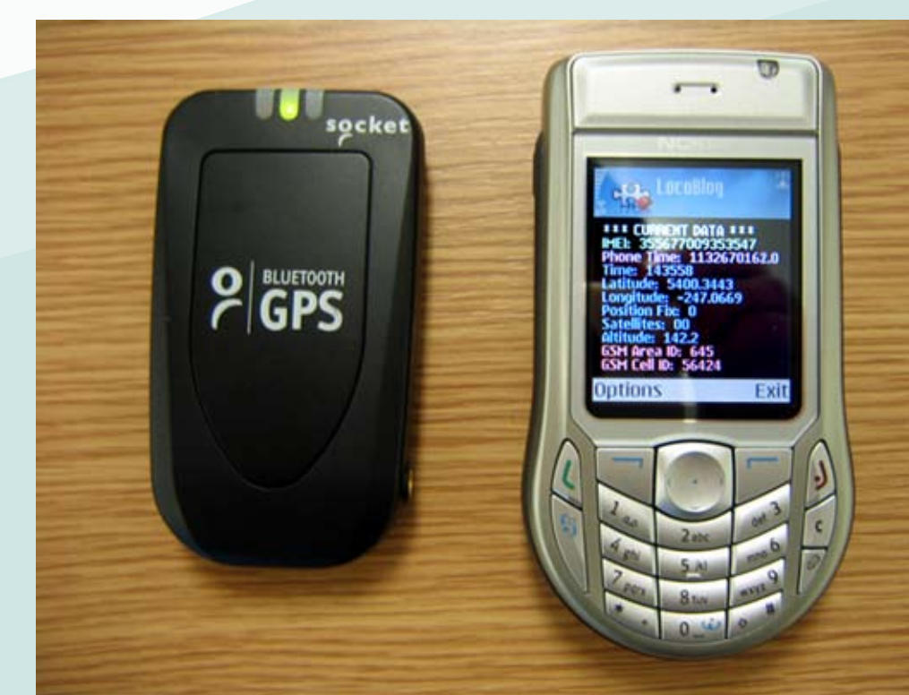
LocoBlog application running on a Nokia 6630 with GPS Bluetooth receiver
